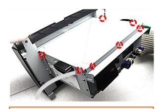
Lead the 20pin picture signal cable out of the housing at the indicated point, without jamming it and fix the housing cover by the 7 screws.
