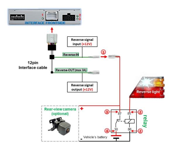
Disconnect the green cable's pre-connected male- and female connectors of the 12pin cable and connect the green input cable "Reverse-IN" to the output connector (87) of the relay.
