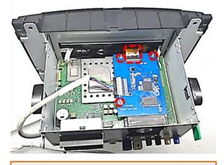
Attach the daughter PCB to the spacers. Connect the previously become free 40-pin copper-coloured ribbon cable to the ribbon cable base "LCD-OUT".
