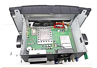
Unclick and disconnect the original copper-coloured 40pin ribbon cable from the ribbon cable base and connect the enclosed 40pin ribbon cable instead.
