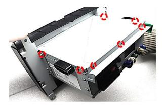
Unscrew the 7 screws at the top of the head unit and remove the housing cover.
