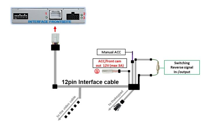
1 The red power supply output ACC/front cam out 12V (max 3A) can be used to power an external source and has a different assignment, depending on the position of dip switch 1 (of 8 dips):
