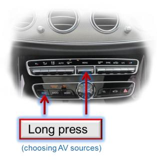
A long press of the NAVI button or the Menu button switches the input from factory mode to the inserted video sources.
