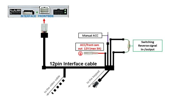
1 The red power supply output ACC/front cam out 12V (max 3A) can be used to power an external source and has a different assignment depending on the position of dip switch 1 (of the black 8 dips):
