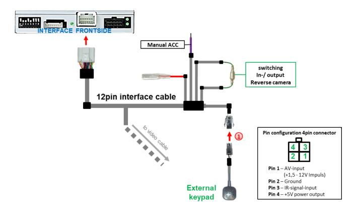
Connect the female 4pin connector of the keypad to the male 4pin connector of the 12pin interface cable.
