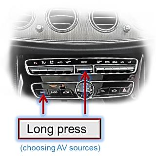
To switch the interface's activated video sources, the factory infotainment's menu or Navi buttons can be used.
