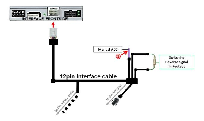
If, after connecting the PNP harness, no interface LED lightens up while the ignition is turned on, the purple coloured wire Manual ACC of the 12pin interface cable has to be connected additionately to ACC or S-contact terminal 86s +12V (e.g. glove compartment illumination).
