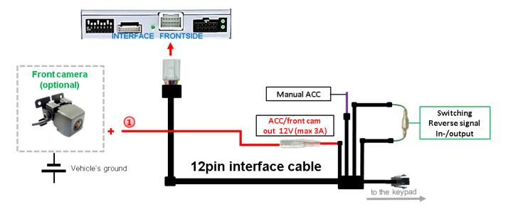
The red power supply output ACC/front cam out 12V (max 3A) can be used to power a front camera. If Dip 1 of the black 8 dips is set to ON, the power supply output gives +12V (max 3A) when reverse gear is engaged incl. 10 seconds delay after reverse gear is disengaged.
