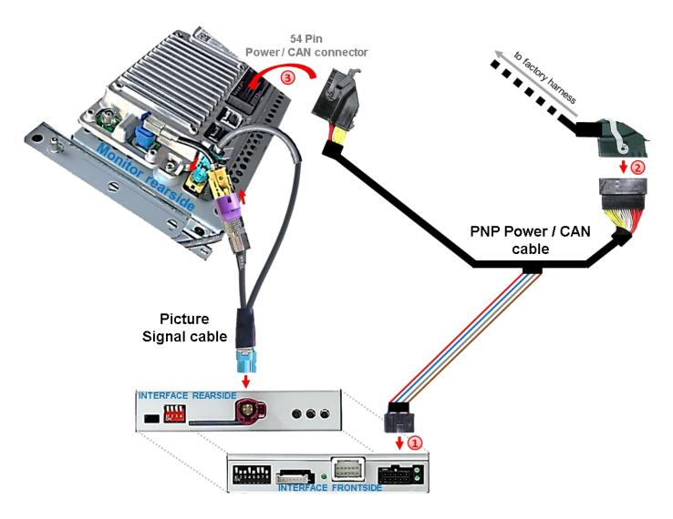
Connect the enclosed PNP Power / CAN cable's female10pin connector to the male 10pin connector of the video interface.
