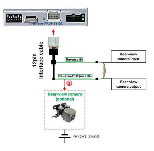
The 12 V power supply for the rear-view camera (max 3A) has to be taken from the 12pin interface cabl's green wire "Reverse-OUT" to avoid an unnecessary, permanent power supply to the camera electronic. Both green cables "Reverse IN" and "Reverse OUT" have to remain connected.
