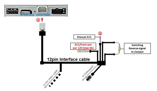
Connect the female 12pin connector of the 12pin interface cable to the male 12pin connector of the video interface.
