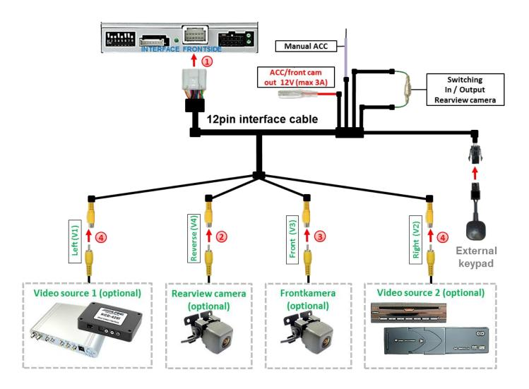
Connect the 12pin interface cable's female 12pin connector to the male 12pin connector of the video-interface.
