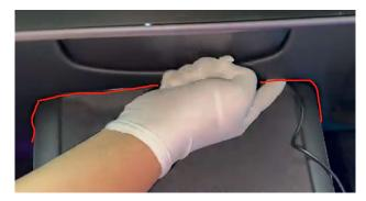
17.Insert the main driver's ambient light cable into the gap as shown in the figure and extend it to the passenger's footwell.
