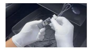
5.Plug the sensor module into the 1to 4 USB port.
