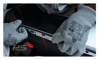
13.Stick the light bar on both sides of the silver trim of the saddle, trying to make it flush with the silver trim.(The light bar is toward the front of the car)
