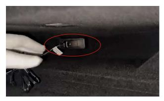
7. Plug the 1 to 4 USB into the USB port of the glove box.
