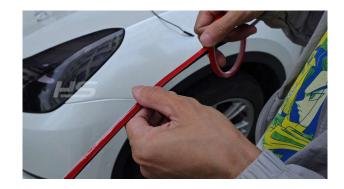
9.Stick the double-sided tape on 1 the center control light strip.
