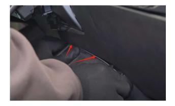
Insert the light bar under the C screen into the gap as shown in the picture.
