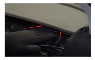
3.Insert the A instrument light bar into the gap above the air outlet.
