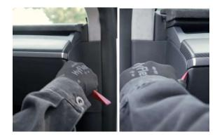
1.Remove the triangular trim panels on both sides of the instrument.
