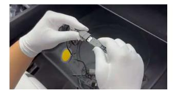
6.Plug the sensor module into the 1 to 4 USB port.
