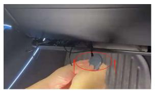
18.Plug the ambient light cable into the one-to-four controller, then wrap the wiring harness and place it on the footwell trim, and finally put the sensor module in with the shiny side facing up.
