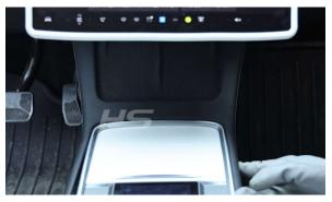
16.Reinstall the wireless charger and plug in the wireless charger.
