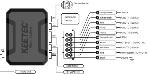
Connecting the system to CAN bus
