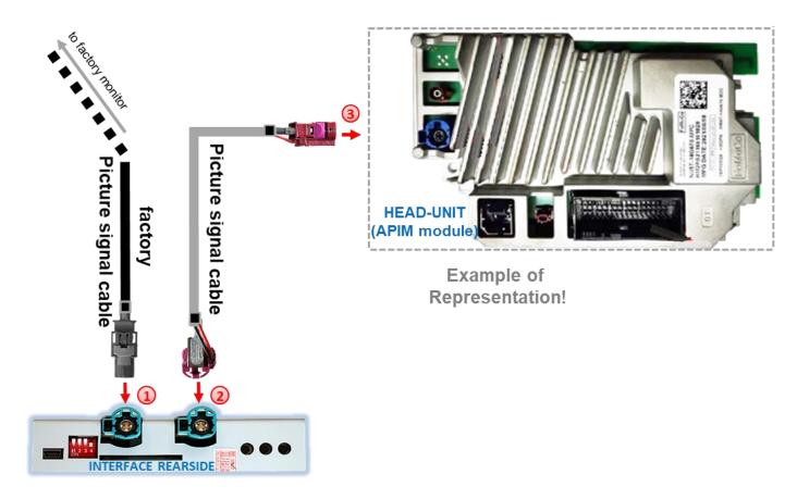
Disconnect the female HSD+2 connector (colours may vary) at the rear-side of the head unit (APIM module) and connect it to the waterblue coloured male HSD+2 connector "**TO LCD"** of the video interface.
