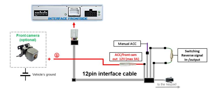
1 The red power supply output Front cam out +12V (max 3A) can be used to power a front camera. If Dip 1 is set to ON (black 8 dips), the power supply output gives +12V (max 3A) when reverse gear is engaged
