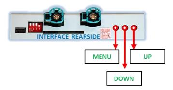
The picture settings are adjustable by the 3 push-buttons at the rear-side of the video-interface. Press the MENU button to open the OSD settings menu or to switch to the next menu item. Press UP and DOWN to change the selected value. The buttons are placed inside in the housing to avoid accidental changes during or after the installation. Picture settings must be done separately for all video inputs while the corresponding input is selected and visible on the monitor.
