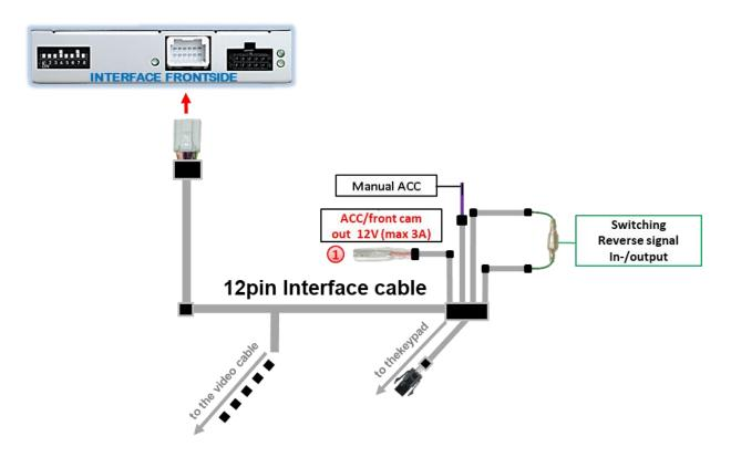
The red power supply output Front cam out +12V (max 3A) can be used to power a front cam with dip switch 1 (of the black 8 dips) to ON.
